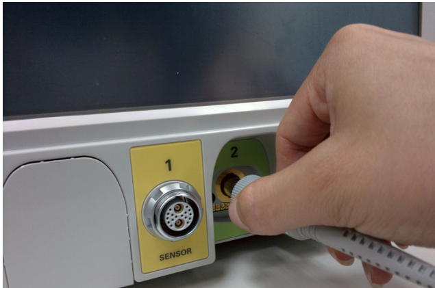
Figure 1-12 Connecting the probe to the 8990B
