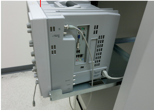
Figure 1-26 Notch at the 8990B to fit the top trim plate
